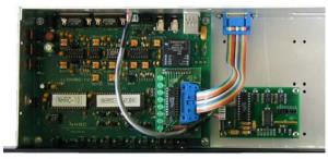
NHRC-10 shown mounted in the NHRC-10/CAB with optional NHRC-10/DOUT and NHRC-DAD boards installed
