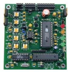
The NHRC-3+ is a new, dramatically improved version of NHRC's popular NHRC-3 Repeater Controller. The NHRC-3+ offers many improvements over the NHRC-3, including simplified programming, a CTCSS input, multitone courtesy tones, a fan control output, four digital outputs and two courtesy tone select inputs.
