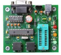
The NHRC-PXP consists of a programmer pod and Windows (tm) based software. They are used together or seperately to program General Electric Phoenix SX, Phoenix SX Scan, and Delta SX radios. (Note: the PXP does not support Delta SX combinations with a "downloading" control head, like S825.)
