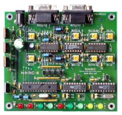
The NHRC-6 is an advanced, low cost dual repeater controller. It has a highly integrated design, using state-of-the-art components, which results in a powerful controller with a low parts count. This increases reliability and lowers cost.
